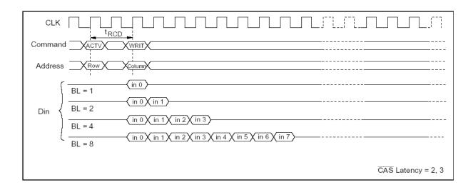
**2. Single write:** A single write operation is enabled by setting OPCODE (A9, A8) to (1, 0). In a single write operation, data is only written to the column address and the bank select address (BA0/BA1) specified by the write command set cycle without regard to the burst length setting. (The latency of data input is 0 clock.)
